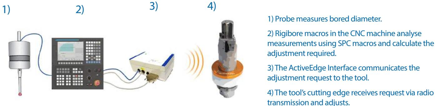
Adjustments can be made to the tool anywhere in the machine after probe data is reviewed, allowing the process to continue.
