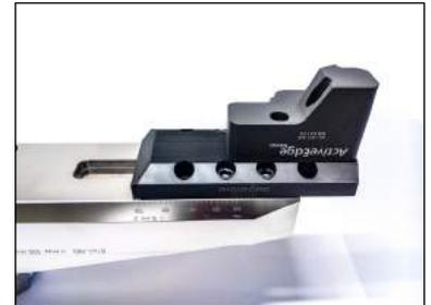
Automatic cutting edge adjustments were delivered through ActiveEdge finish cartridges in the Nexus module.
